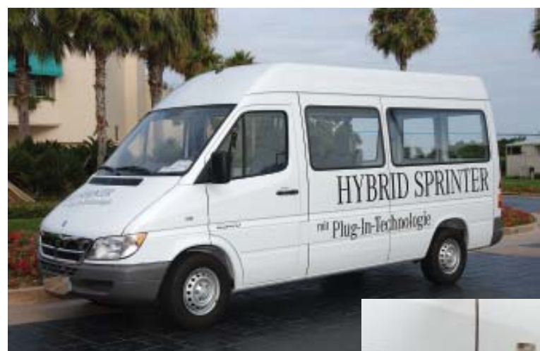
This Dodge Sprinter Plug-in hybrid van, being tested in the U.S., is one answer to conserve petroleum and reduce imports from overseas. Plug-in hybrids can be recharged in standard electric sockets with 70 cents per gallon (gasoline equivalent) of electrical energy and then be driven 20 to 60 miles without using gasoline.
