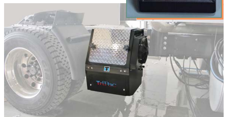
Some states have anti-idling laws. An on-board auxiliary power unit (APU) like this can save 80 percent on rest-stop fuel expenses, reduce engine hours, maintenance costs, and driver fatigue. Cabin HVAC, battery charging and engine warming can be powered by the APU when the truck engine is shut down.
