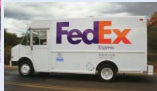
FedEx partnered with Environmental Defense and Eaton to build this diesel powered hybrid-electric step-van which achieves remarkably low emissions and excellent fuel economy.
