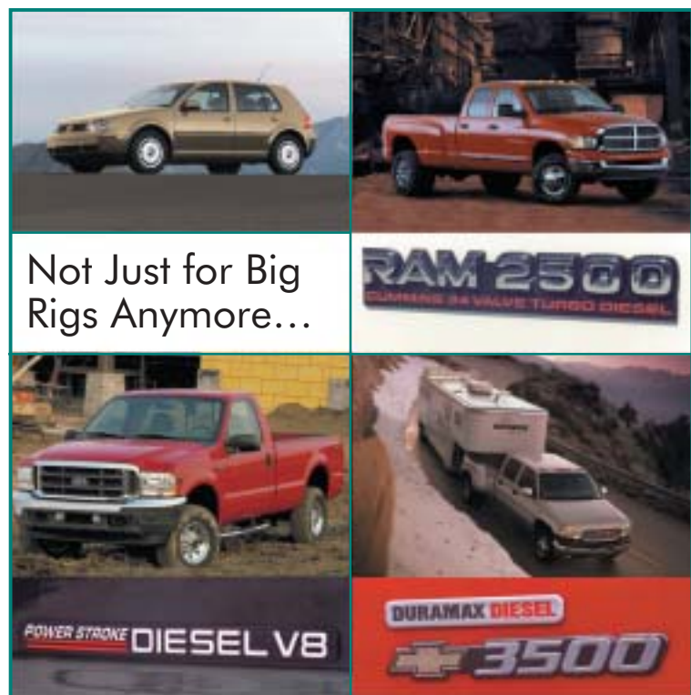
VW started the light-duty diesel revival with its modern 1.9 liter 4 cylinder turbo-diesel direct injection (TDI) engine, used here in the Golf. Also shown: Dodge Ram with Cummins 24 valve diesel; Ford HEUI Powerstroke; and GMC Duramax 6.6 V8 applications.
