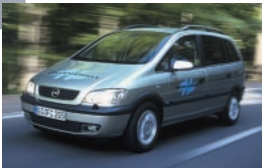
GM's HydroGen I is a good example of a fuel cell hybrid electric vehicle. It runs on liquefied (cryogenic) hydrogen and the emits only water and oxygen.
