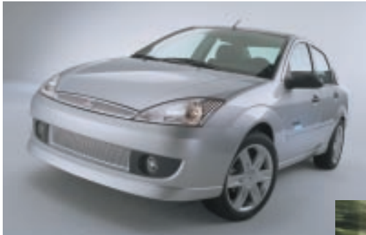
Ford's Focus FC-5 sedan is fueled with methanol. It's a 2000 model prototype FCV.
