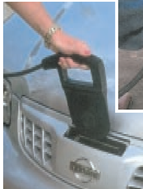
The jury is still out on which of these SAE-approved charging connectors will be accepted by users: inductive "paddle" (l) or conductive connector (r).
