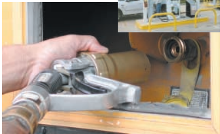
Refueling a propane vehicle is quick and easy: the standardized 'no-bleed' nozzle screws in place for emission-free fueling.
