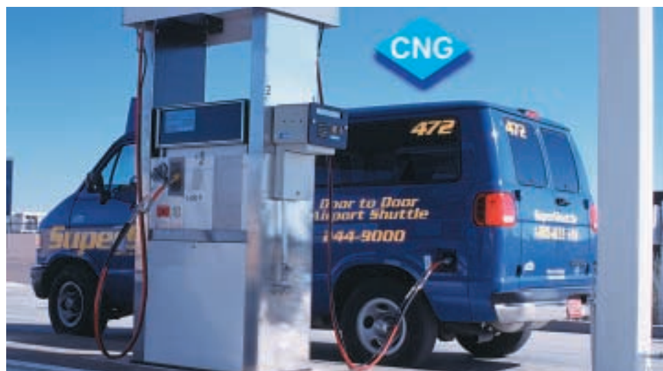
"Fast-fill" compressed natural gas (CNG) refueling is as easy and as quick as gasoline refueling. This airport passenger van is typical of the vehicles best suited for alternate fuel use- it is centrally refueled, travels local routes, and racks up high mileage. Note the CNG diamond which must be displayed on the rear of the vehicle. Watch for similar emblems required on LNG and Propane powered vehicles as you travel the nation's highways.
