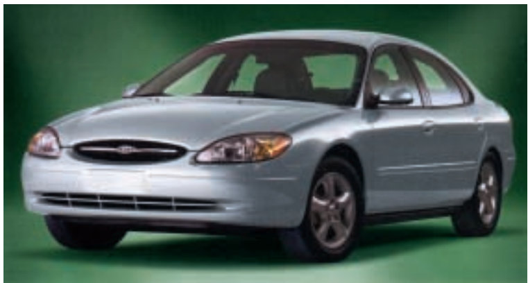
This Ford Taurus flexible fuel vehicle (FFV) comes with the 3.0L V-6 engine and runs on ethanol (E85), gasoline, or any combination of the two fuels.
